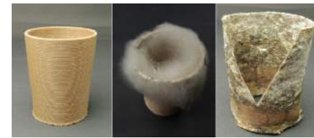
3) left: fresh printed GROWLAYbrown middle: cotton-like mold growth right: slow-growing lichen
