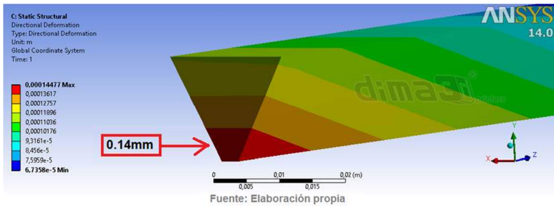
Figure 13. Deformation caused by internal tensions printing with Dimafix® at 90°C (194°F)
